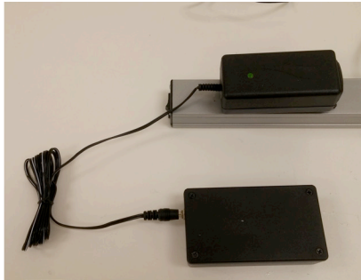
Battery fully charged - Green LED
